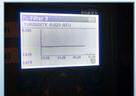
Filtered water quality is continuously monitored and recorded to ensure production meets compliance standards. The SCADA system received new turbidity units, controllers and upgraded software. This system allows operators to monitor production and alerts them of needed operational changes.
